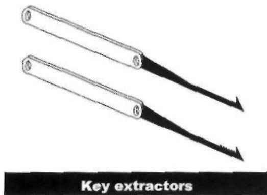
As the name implies, the key extractor is used to remove broken key segments that are still stuck in the lock's keyway. They are usually hook shaped, or have one-way teeth that allow it to be inserted easily, and can grip and pull the obstructing object out.
