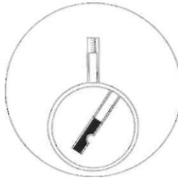
**Front view—key inserted & plug rotated**
