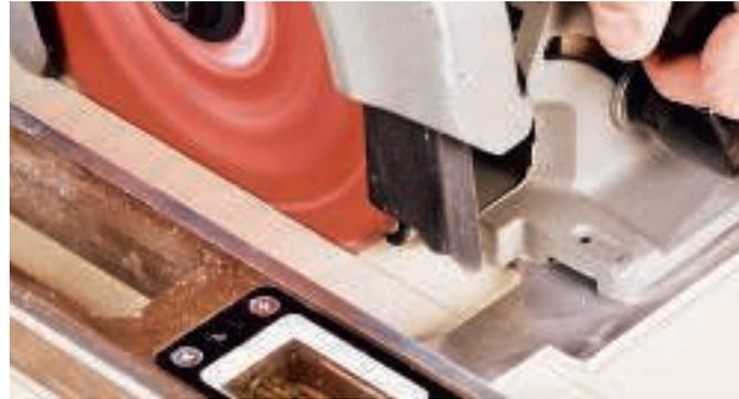
A careful cut along a scored line greatly minimizes splintering. Always use a straightedge guide to keep your saw straight during this cut.
