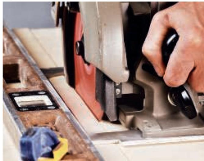
Using a straightedge with a circular saw
