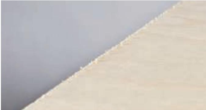
Crosscuts made with a circular saw are notorious for splintering face veneers.
